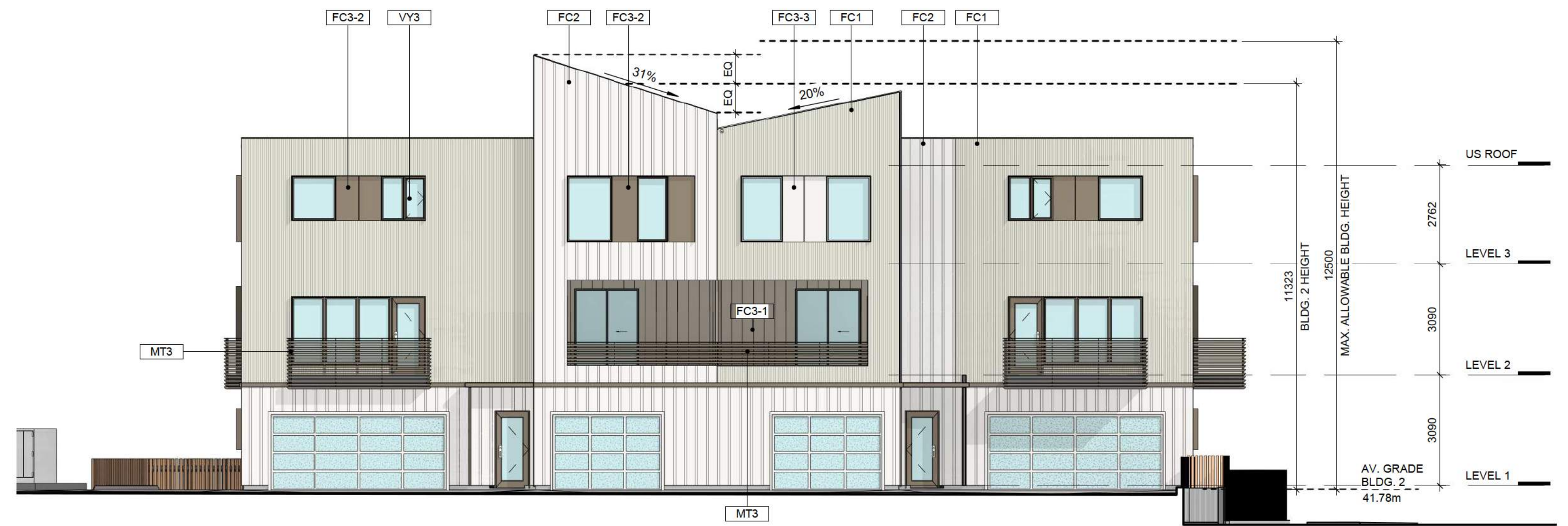
2 Elevation Bldg. 2 North. SCALE = 1 : 100
