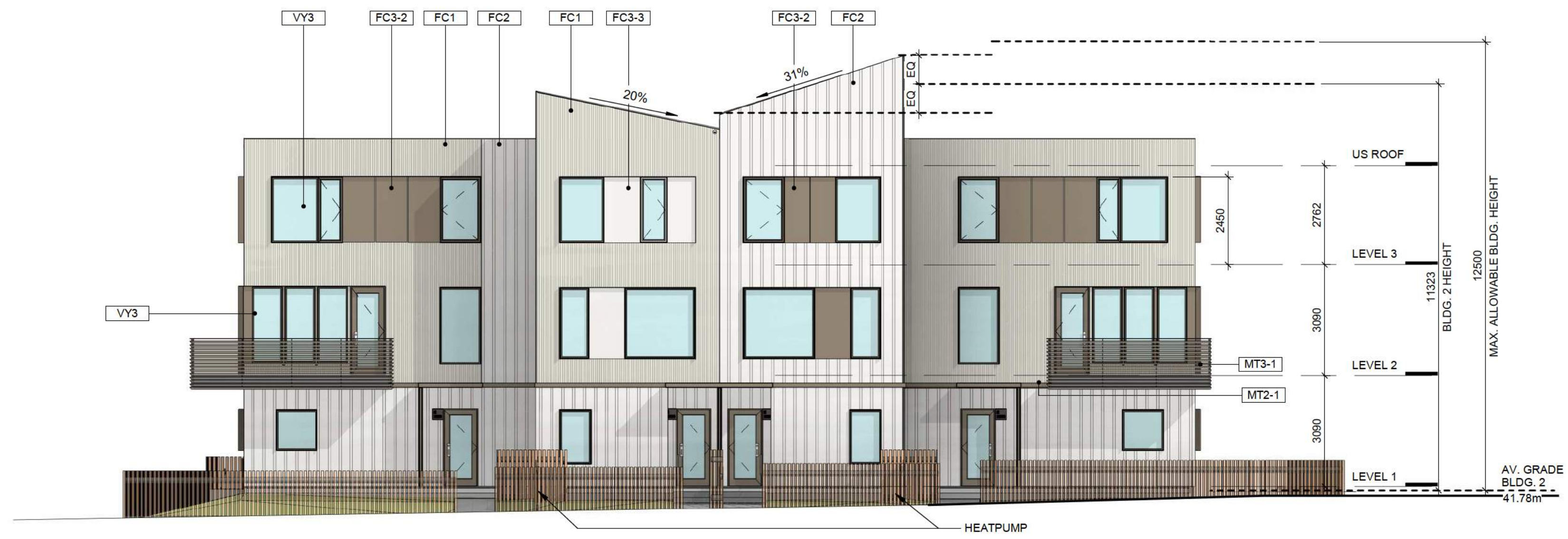
1 Elevation Bldg. 2 South. SCALE = 1 : 100
