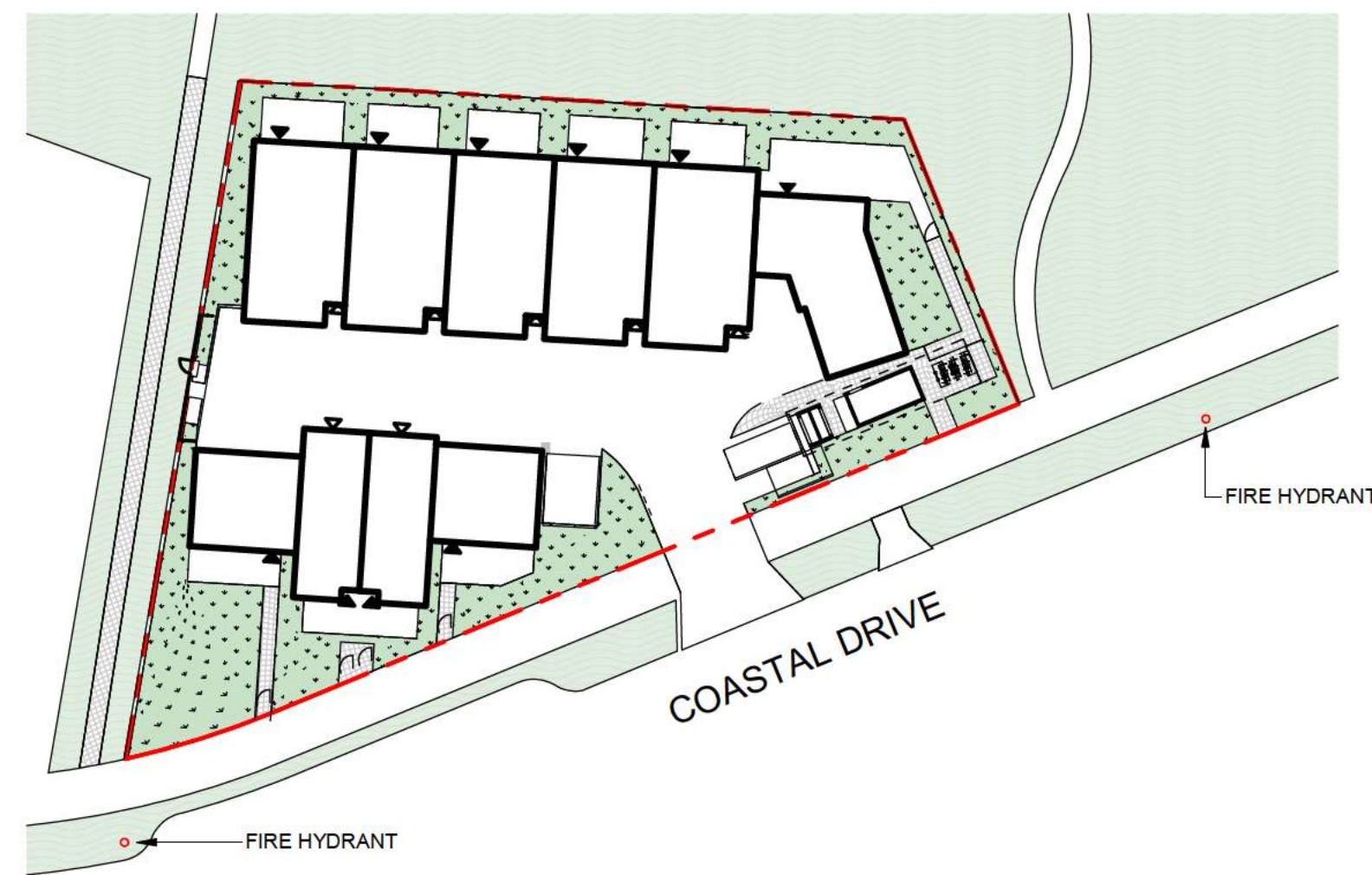
6 Fire Hydrant Location. SCALE = 1 : 500
