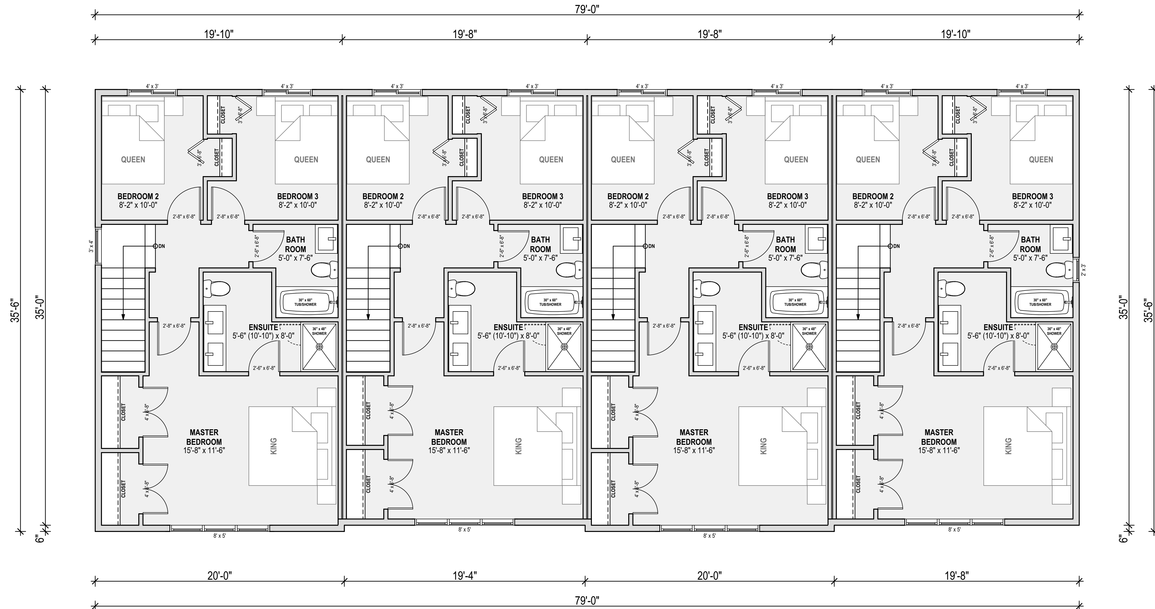
1 A15 UPPER FLOOR PLAN SCALE 1/4" = 1' CEILING HEIGHT: 9'-0" FLOOR AREA PER UNIT: 704.17 sq/ft
