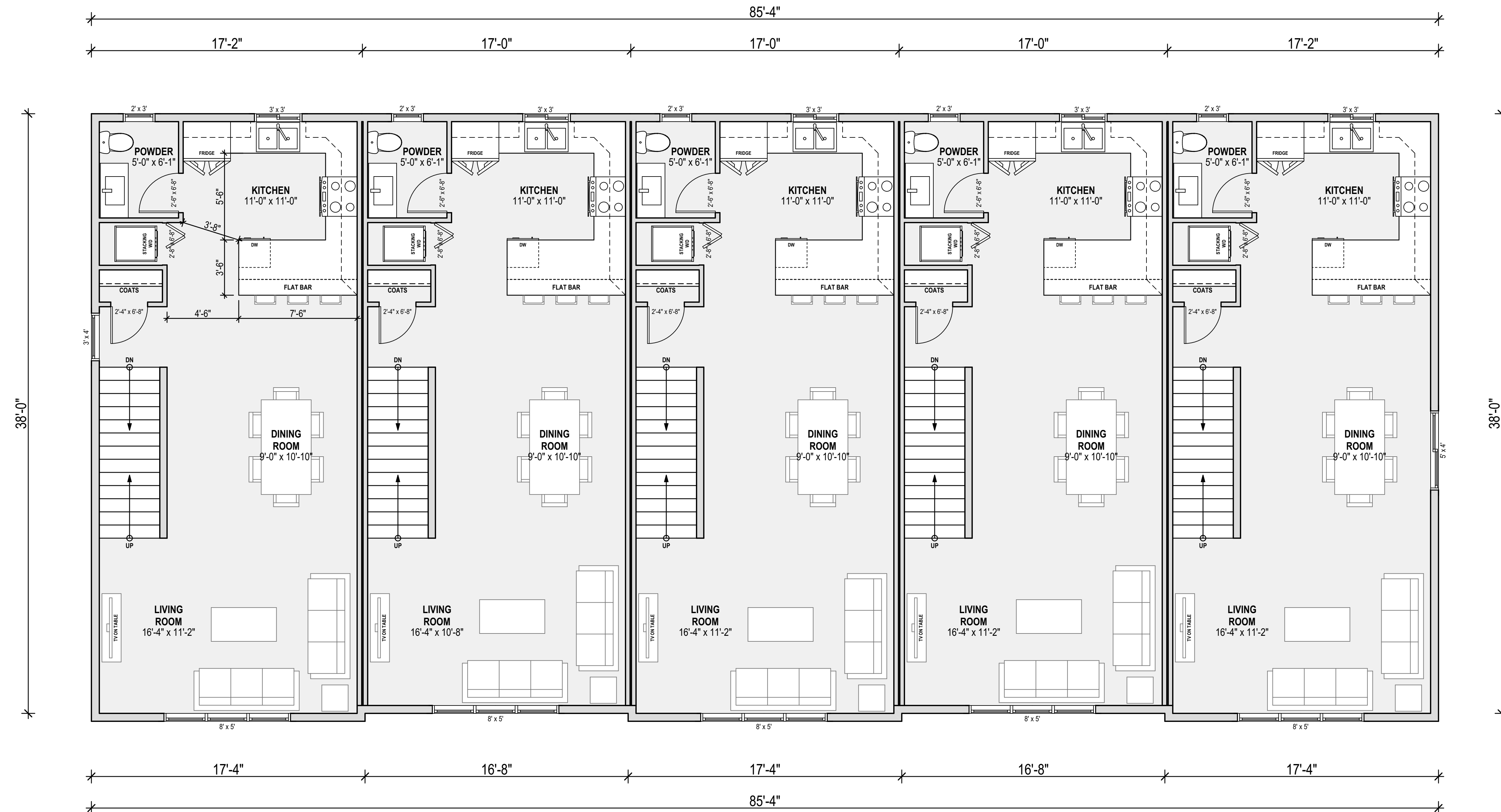
1 A10 MAIN FLOOR PLAN SCALE 1/4" = 1' CEILING HEIGHT: 9'-0" FLOOR AREA PER UNIT: 652.33 sq/ft
