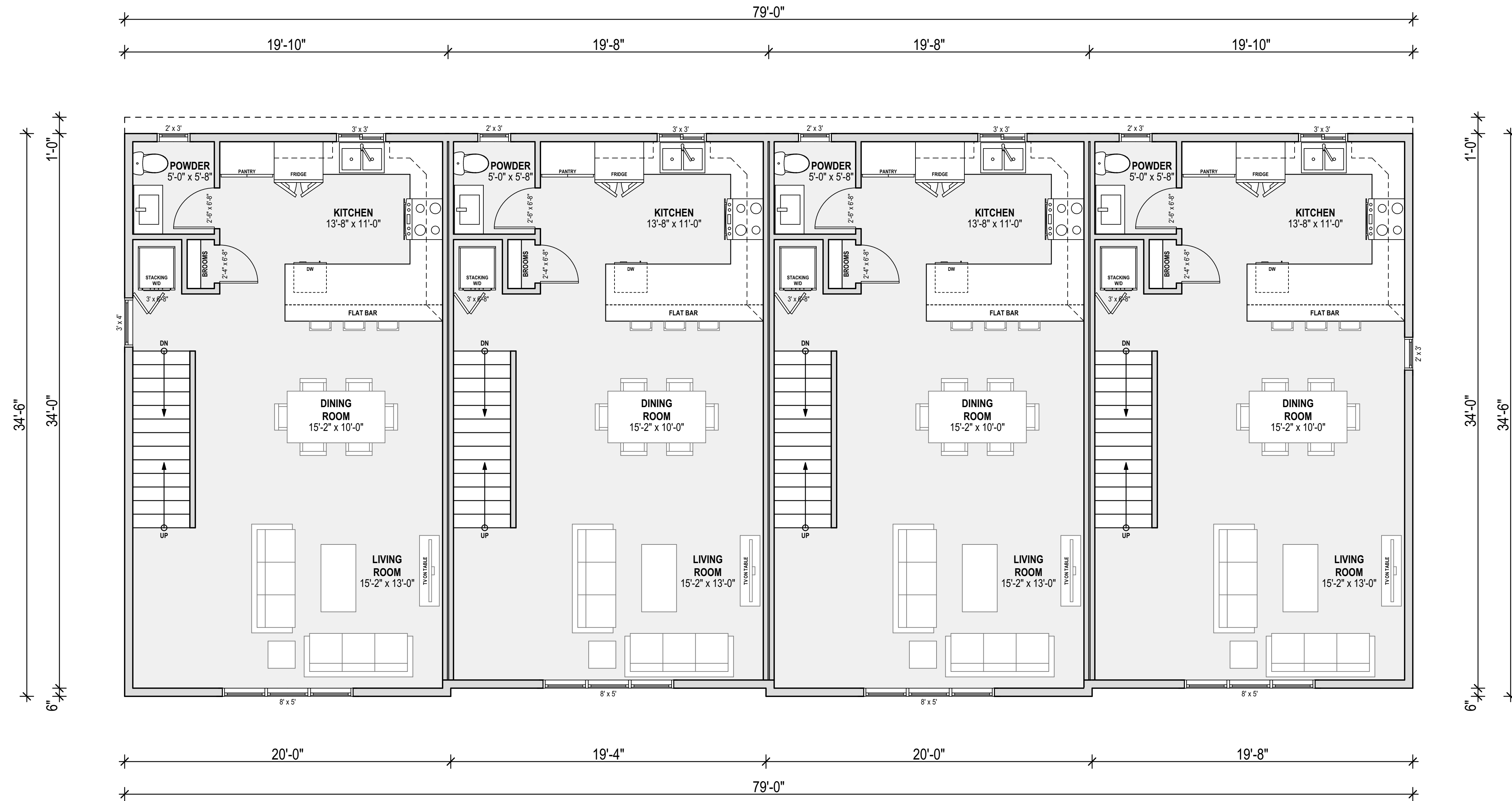
1 A14 MAIN FLOOR PLAN SCALE 1/4" = 1' CEILING HEIGHT: 9'-0" FLOOR AREA PER UNIT: 684.24 sq/ft
